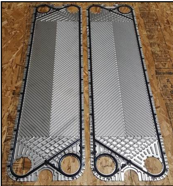
Figure 18 – Directional Flow Plates
