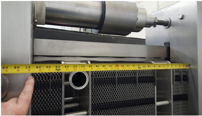
Figure 30-Tightening Dimension for a Plate Heat Exchanger
