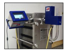
CCT 4.0 Installed on heat exchanger testing for internal defects
