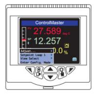
Operator level menus are used to adjust setpoint(s) and output(s), select setpoints, select the view and to enter *Basic* and *Advanced* modes (via the *Access* level) – see page 27.
