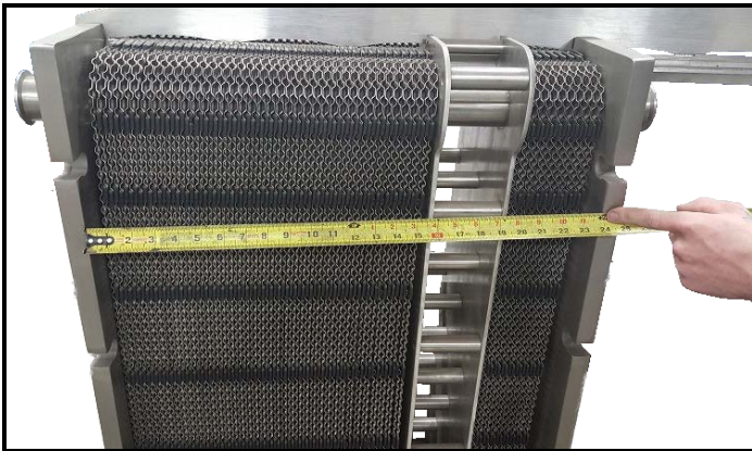
Figure 25 – Tightening dimension for a Plate Heat Exchanger
