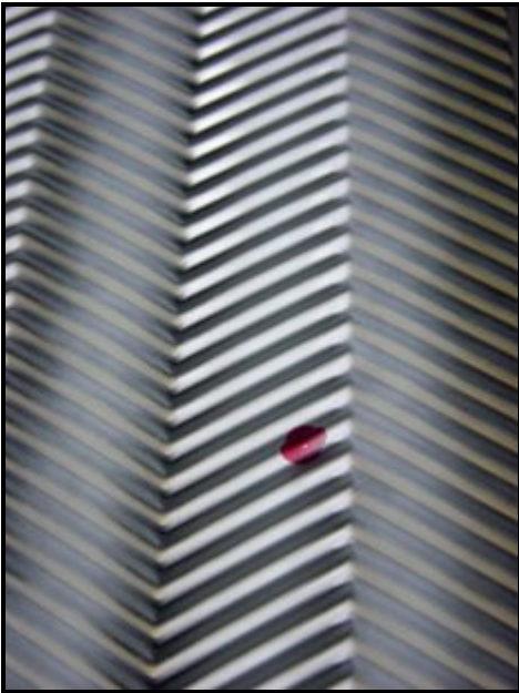
Figure 28 – Results of a Plate Dye Test
